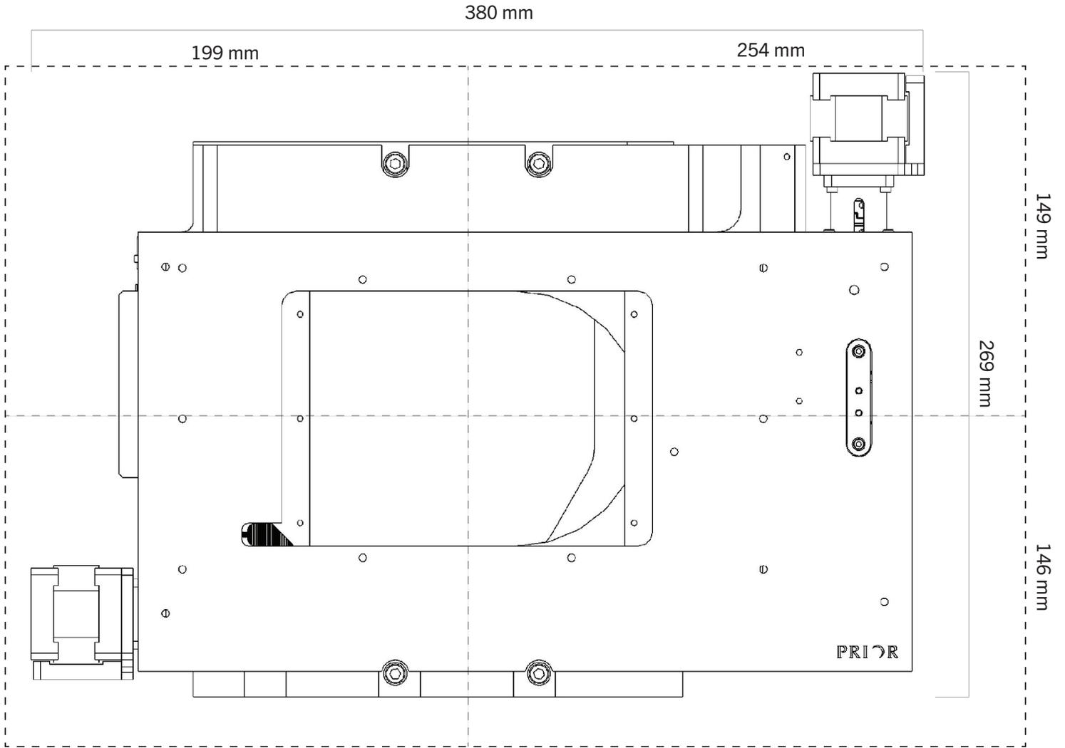
\*Outer dotted line shows the maximum footprint of the stage when at the limits of travel.
