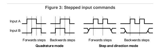
To ensure the controller can be easily integrated with other systems, this is also configurable to reverse direction, and for step and direction mode to trigger on rising or falling edge.
