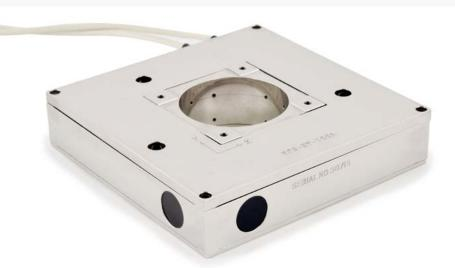
The NPS-XY-100A and the NPS-XY-100A-UHV NanoMechanisms are piezo scanned flexure guided stage with integrated capacitance position sensors capable of sub- nanometer resolution and reproducibilty. The NPS-XY-100A-UHV has been designed to operate down to 10-9 Torr.
