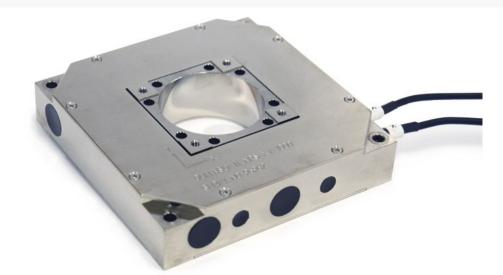
The NPS-XY-100D NanoMechanism is a piezo scanned flexure guided stage with integrated capacitance position sensors capable of sub-nanometer resolution with market leading dynamic performance.
