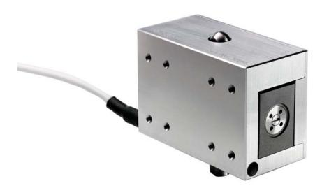
The NPS-Z-500B-UHV delivers over 100um full range at 80K at 10-9 torr. The stage is designed to operate in closed loop mode using capacitive positioning sensors. The advanced flexure design results in a highly linear device with outstanding resolution, repeatability, stiffness and stability. Low off-axis errors and a high resonant frequency further enhance the performance of this advanced design.
