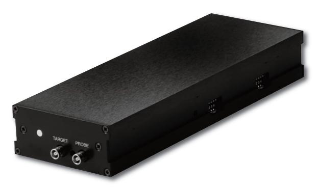
The NS2000 is a single channel stand-alone electronic module for driving the NX and NC NanoSensor series. It operates by measuring the change in capacitance of a parallel plate capacitor and outputs an analogue voltage proportional to the NanoSensor gap.
